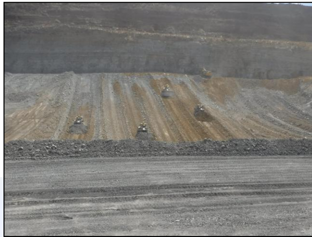
Figure 10 – Bulk push operation.
