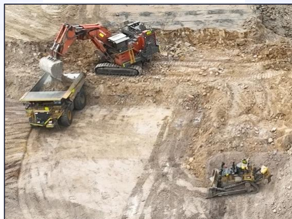
Figure 7 - Example of good position for dozer to wait.
