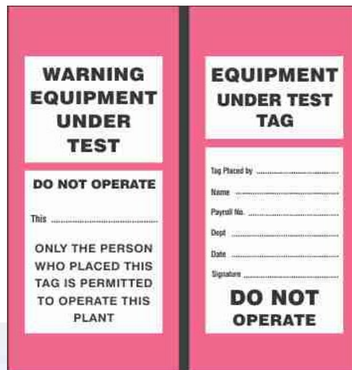
Figure 6 : Equipment under Test Tag
