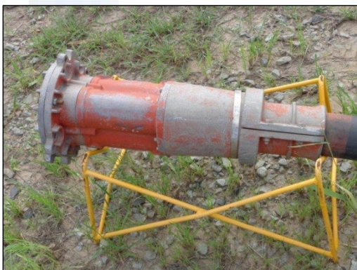
Figure 2: 11Kv HV Plug
