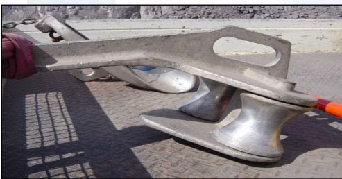
Figure 12: Cable Relocation Roller
