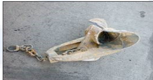
Figure 13: Cable Handling Puller
