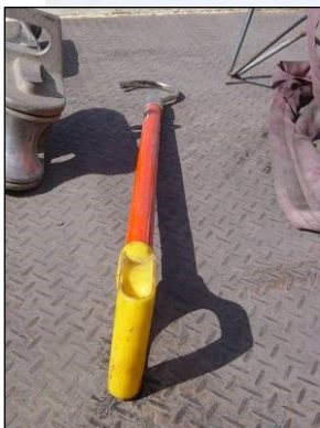
Figure 4 Cable Handler – hand tool (used to make small adjustments where excessive force is not required).
