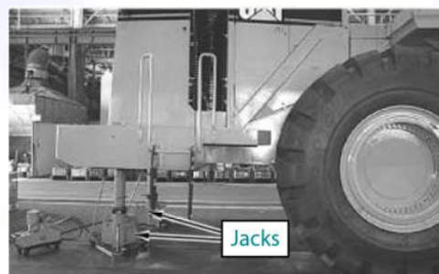
Figure 8 Jacking machine's rear.
