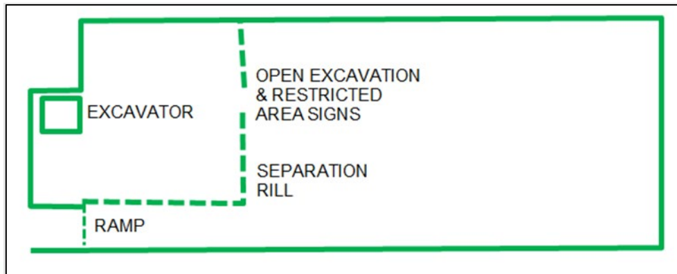
Figure 4 : Accessing a bench from the front of an excavator.
